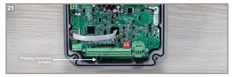
Connect the fire suppression system wires from the dry contacts on the relay to terminals COM and DI2. Route the fire system cable out via the provided strain relief.
