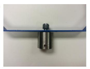
4. Attach Oscillator Linkage Bolt to Oscillator Arm. Tighten Nut on to bolt as far down as possible.
