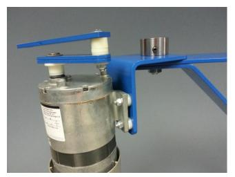
Attach the Yoke Bearing Assembly to the bottom of the supplied yoke. Toque Nut to 100 foot pounds.
