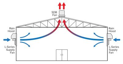
Use roof exhausters in conjunction with supply fans to remove warmer air, fumes, and vapor.
