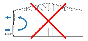
An example of a *poorly* setup system. Air flows in and out of the same area, resulting in no air flow for the rest of the building.
