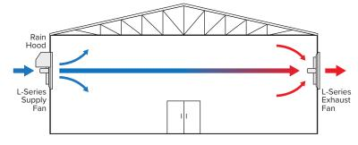
If no dock door is present, position supply fans on opposite wall of exhaust fans. Supply fans should be on the north side of the building so as not to bring in heat from the sun.
