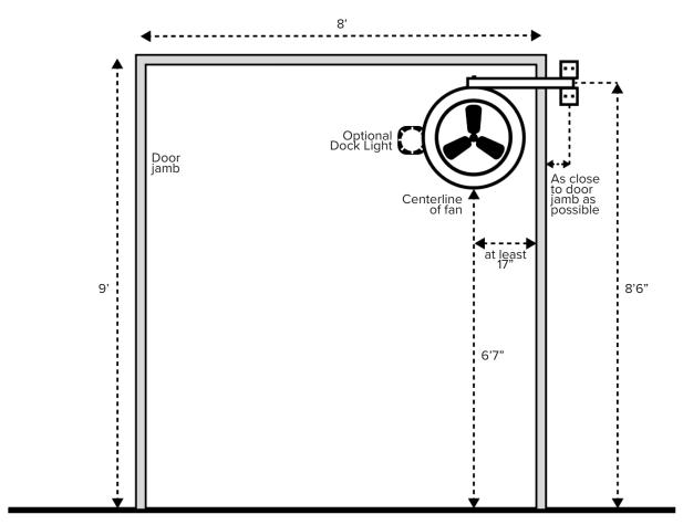
**Note:** The TC-18 is designed to purge a trailer of hot air. Mounting in the top corner pushes air through the trailer and out the opposite corner of the door, as shown below, with an exit velocity of approximately 200 FPM. The fan will not be as effective if positioned other than what is recommended or by directing on an individual.
