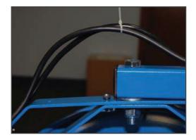
5. Install 5/16" nut and bolt into hole next to 5/8" bolt opposite of the arm. This prevents over rotation of the fan and damage to power wiring.
